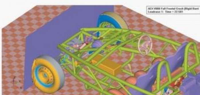
Full frontal crash with rigid barrier
